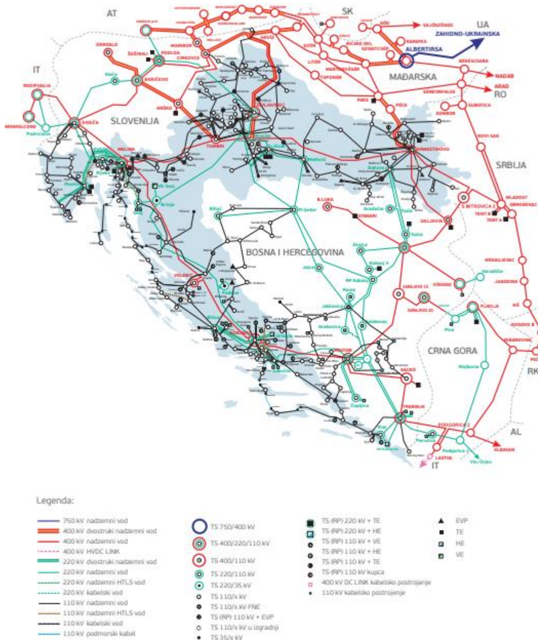
Figure 4-17 Croatian electricity system transmission grid with surroundings
