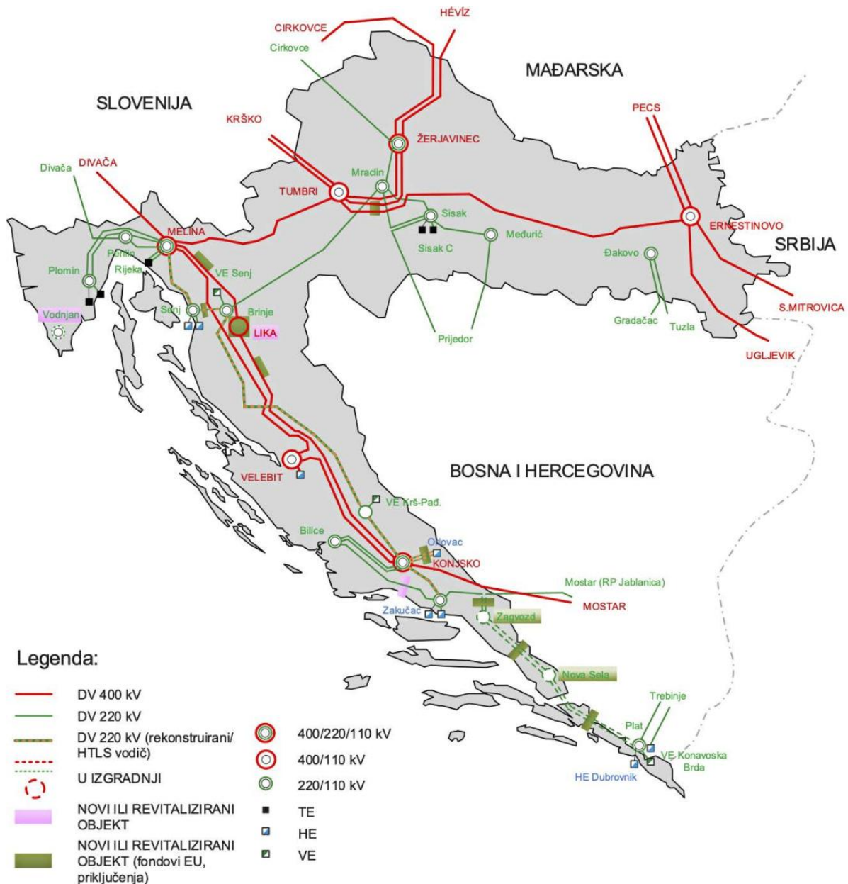
Figure 4-20 Foreseen topology of 400 kV and 220 kV grid on the territory of the Republic of Croatia in 2031
